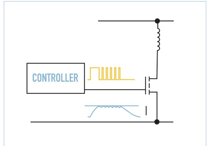
When a phase winding is first energised, the controller initially switches on for a period sufficient to attain the rated phase current, it then switches alternately on and off at a duty cycle which maintains this current level.
