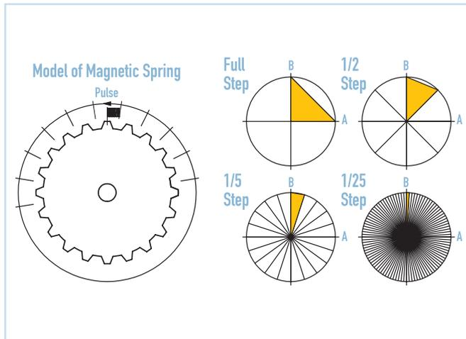
In the above diagrams, the yellow shaded area represents the energy input to the spring/mass system in each step with full-step drive, and at fractional step drive for different resolutions. This energy pulse is closely related to the tendency to resonance.
