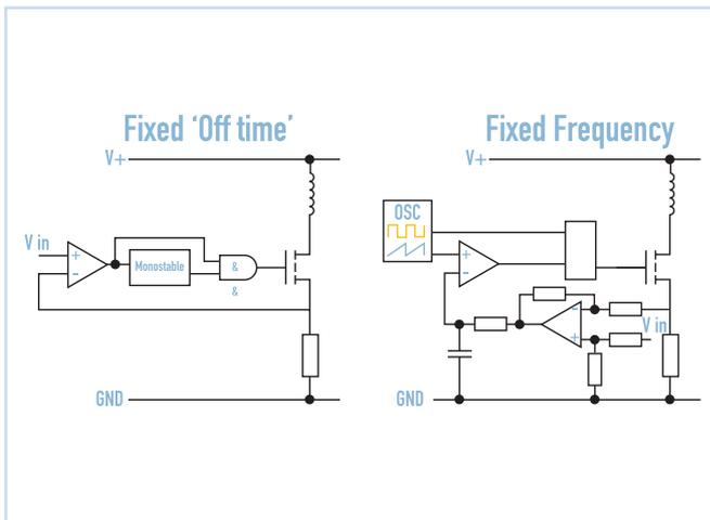
In the 'fixed off-time' drive, the winding current is measured and compared to a target value. When this exceeds the target, a monostable causes the output to switch off for a short fixed interval. This interval is sufficient for the current to decay below the target value, so when the 'off-time' is finished, current again rises and the cycle repeats. A small ripple is seen in the current waveform about the target value.
