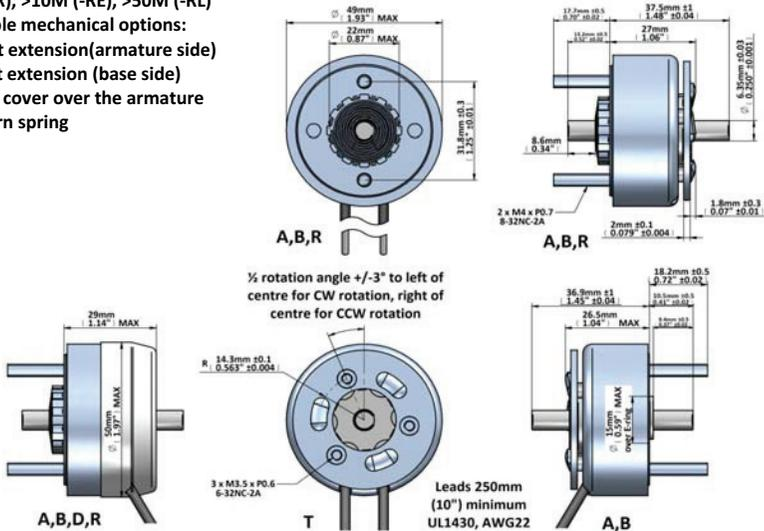
Data at 20°C, device connected to heatsink 190x190x3mm aluminum return spring 26 ~ 35 mNm
