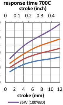
Data at 20°C, device connected to heatsink 390x390x3mm aluminum
