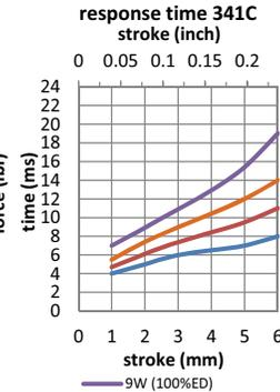
Data at 20°C, device connected to heatsink 120x120x3mm aluminum
