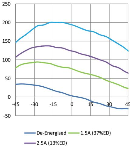
Response (ms) vs Load Inertia (gcm<sup>2</sup>)
