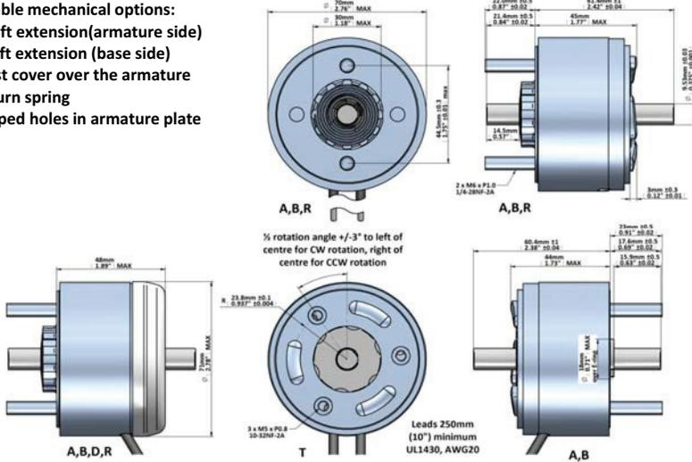
Data at 20°C, device connected to heatsink 390x390x3mm aluminum return spring 75 ~ 105 mNm
