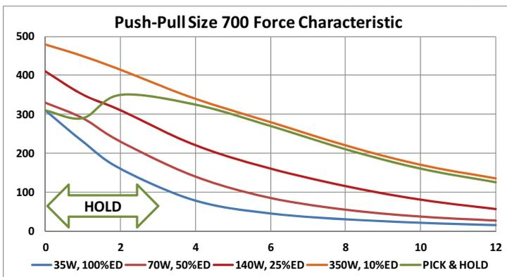
at different excitation power showing greater force with increasing excitation power, and the shape of the curve with force increasing as displacement reduces towards zero are similar for most linear solenoids), the use of a pick and hold circuit enables force to be realised at the extended position similar to an intermittent duty curve, with continuing excitation power comparable to (or even lower than) that of the 100% duty curve.
