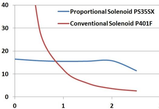
As the excitation current increases, the force developed by the solenoid increases. The solenoid plunger pulls in until the magnetic force is balanced by the opposing spring force. As the current is increased, it will pull in further to attain a new equilibrium position. In this way, a system is realised in which the position is proportional to the applied excitation current. As a simple analogy,
