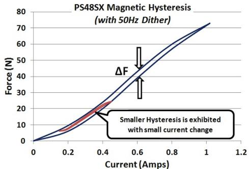
Hysteresis losses will limit the precision to which force or position can be accomplished using a proportional solenoid. Mechanical hysteresis will vary for different bearing types, for dry / maintenance free bearings it will typically be 10-20% of the developed force, for lubricated bearings, or for flexure supports it can be smaller.
