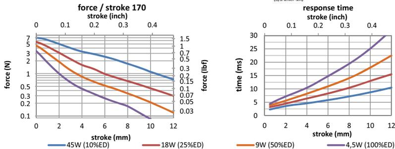
Data at 20°C, device connected to heatsink 50x50x3mm aluminum
