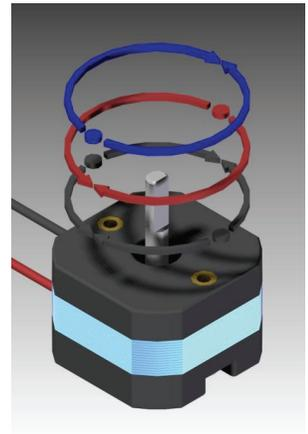
The mechanical limit stops restrict rotation so the device cannot turn all the way to the equilibrium
