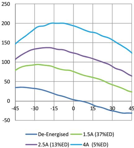
Response (ms) vs Load Inertia (gcm<sup>2</sup>)
