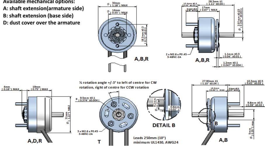
Data at 20°C, device connected to heatsink 90x90x3mm aluminum return spring 5,5 ~ 9 mNm
