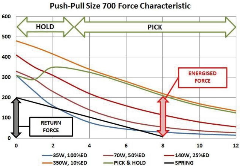
Latching (also known as bistable or self-holding) solenoids facilitate the same force and speed benefits that can be achieved through the use of a pick and hold drive configuration, but with simpler drive requirements. These devices also exhibit lower inductance in the energised position than conventional solenoids due to the properties of the permanent magnets employed in their construction. Latching solenoids are not generally suitable for use in applications requiring 'fail-safe' operation.
