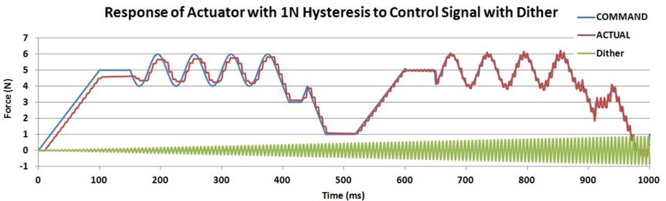
As the amplitude of the dither signal increases, the deviation of the 'ACTUAL' force from commanded value will reduce, reaching a minimum when the peak-to-peak amplitude of the dither signal corresponds to the solenoid hysteresis. If dither amplitude is increased further, the solenoid will begin to exhibit some oscillation about the commanded value.
