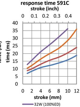
Data at 20°C, device connected to heatsink 310x310x3mm aluminum
