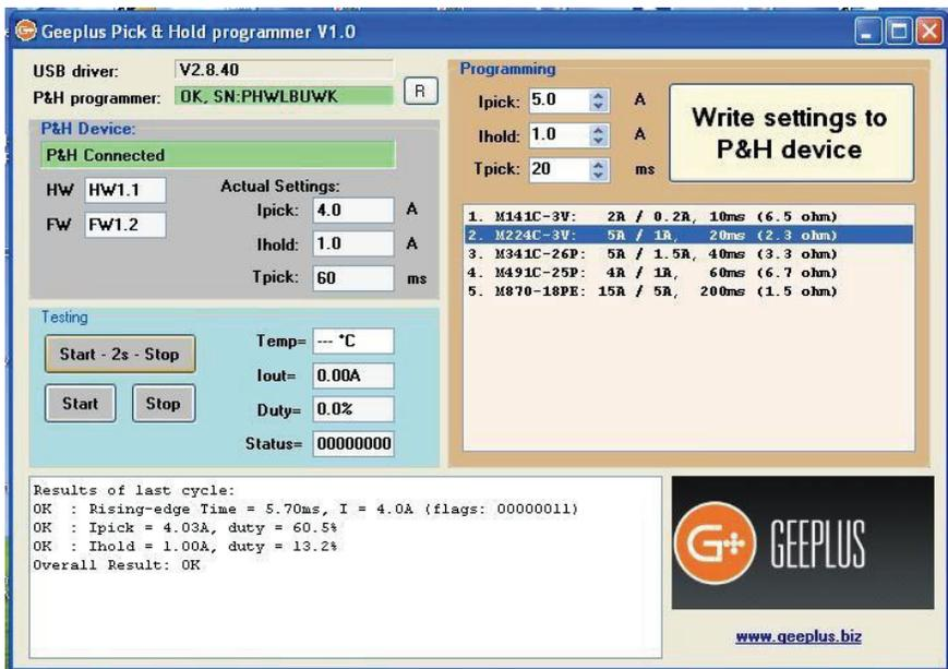
As it opens up, the programmer defaults to the smallest values for safety, you can pick a device of appropriate size as a starting point, press the button 'Write Settings to P&H Device' to store these settings in the module.
