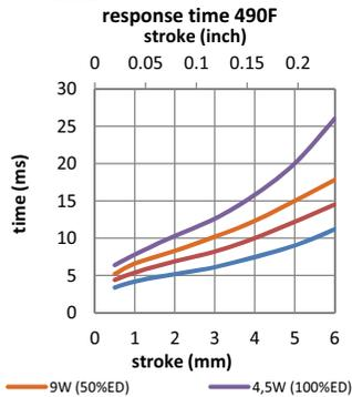
Data at 20°C, device connected to heatsink 190x190x3mm aluminum
