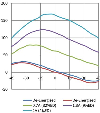
Response (ms) vs Load Inertia (gcm<sup>2</sup>)
