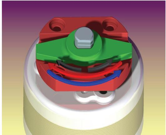
A pulse of electrical power applied in the reverse direction, will cause the solenoid to develop torque acting in the counter-clockwise direction, and to turn in this sense until it comes to rest against the stop. This excitation condition is represented by the blue arrow. If power is then removed the detent torque will cause the solenoid to remain in this position.
