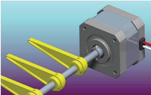
The solenoid incorporates bearings to support the shaft of diverter mechanism on one side of the machine, and is designed for simple assembly where the solenoid is fitted over the end of the diverter shaft, and engages with a roll pin fitted through the shaft to transmit torque.
