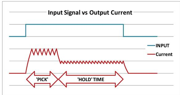
The PHu modules can be used to implement control of large solenoids in an end-user application, the user-friendly interface also makes them a superb development tool to explore the maximum performance achievable from a wide range of solenoids during product development.
