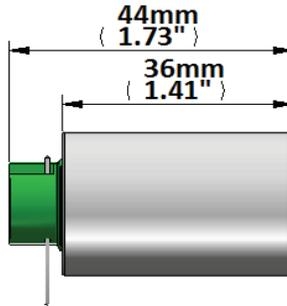
This part does not include bearings - guidance should be provided in customer application to maintain clearance between coil and magnet assembly
