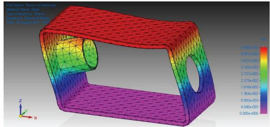
the image [animation in powerpoint presentation] shows in exaggerated form how the frame distorts when the plunger impacts the end stop of the solenoid, under repeated cycles the frame may fatigue and break, typically at the staked joints, or bends in the frame. This mode of failure is more likely to occur with large parts operating at high force and with heavy loads.
