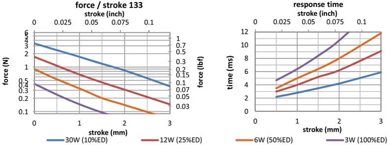
Data at 20°C, device connected to heatsink 50x50x3mm aluminum
