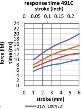
Data at 20°C, device connected to heatsink 190x190x3mm aluminum
