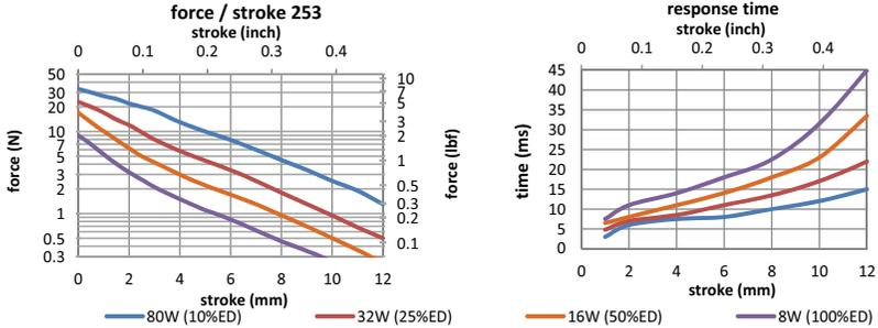
Data at 20°C, device connected to heatsink 100x100x3mm aluminum
