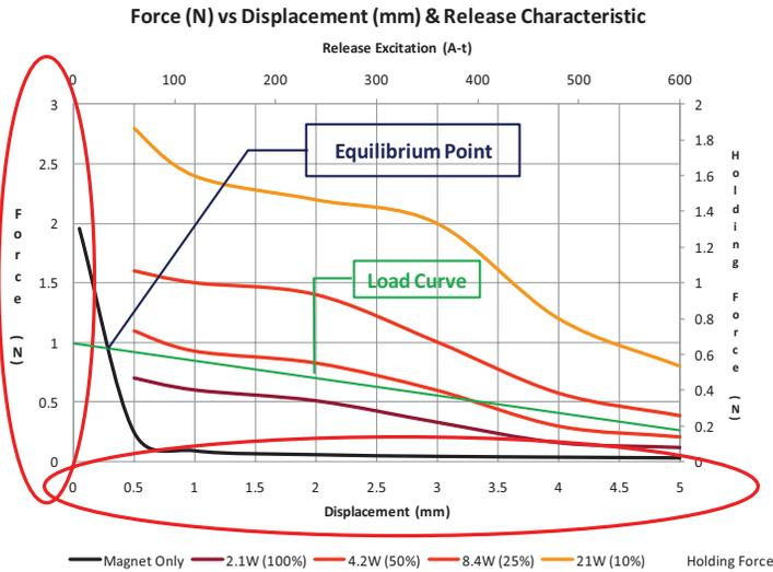
When the latching solenoid is energised with current in the forward direction, the excitation of the coil induces magnetic flux reinforcing the field due to the permanent magnets. As the excitation current increases, the force developed increases.
