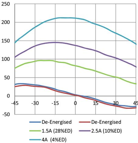
Response (ms) vs Load Inertia (gcm<sup>2</sup>)
