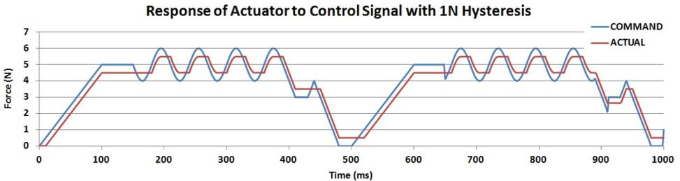
The 'COMMAND' line represents the force developed by a perfect solenoid, without friction or magnetic hysteresis. The 'ACTUAL' line represents the force that would be measured in practise at the output shaft of the device.
