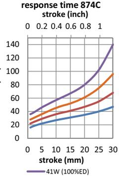
Data at 20°C, device connected to heatsink 520x520x3mm aluminum
