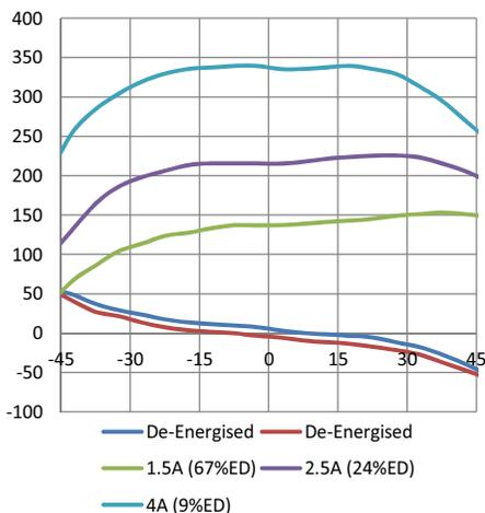
Response (ms) vs Load Inertia (gcm<sup>2</sup>)
