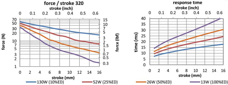
Data at 20°C, device connected to heatsink 130x130x3mm aluminum
