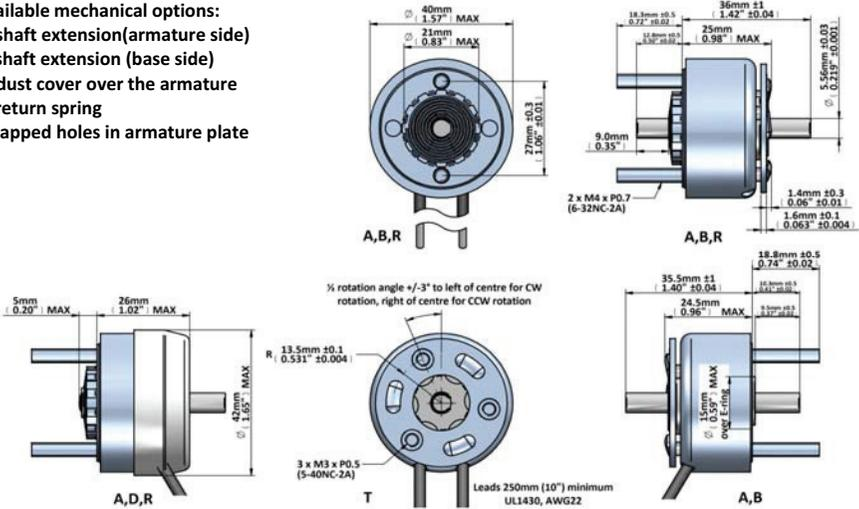
Data at 20°C, device connected to heatsink 160x160x3mm aluminum return spring 16,5 ~ 24 mNm
