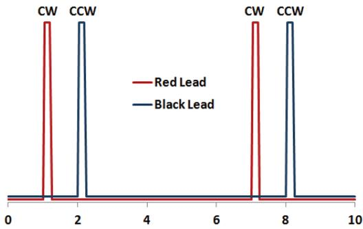
By closing either S1 and S4, or S2 and S3 while the other switches are open, the current can be caused to flow through the solenoid coil in either the forward or the reverse direction. With momentary excitation pulses as depicted in the timing diagram the solenoid can be driven CW or CCW, remaining in either position with no power applied in between.
