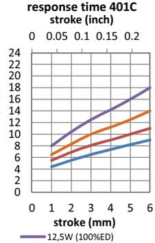
Data at 20°C, device connected to heatsink 160x160x3mm aluminum
