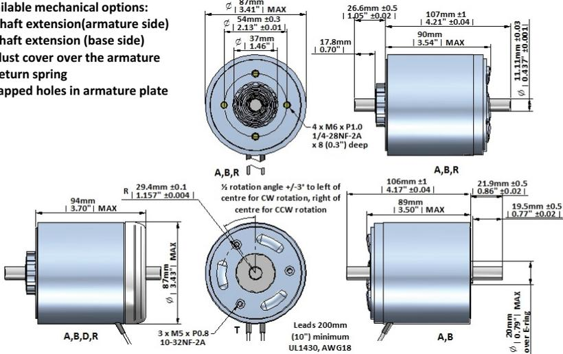
Data at 20°C, device connected to heatsink 520x520x3mm aluminum return spring 190 ~ 140 mNm
