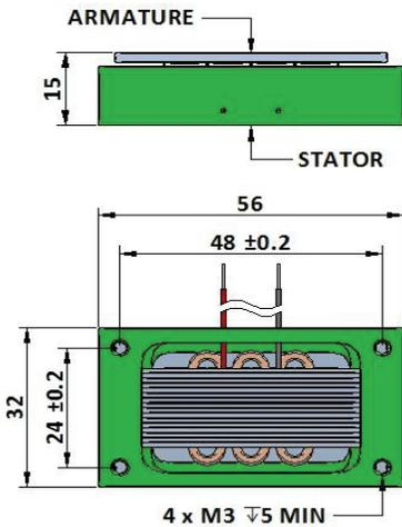
**AIRGAP 0.8 ± 0.2 MUST BE MAINTAINED BETWEEN STATOR AND ARMATURE**
