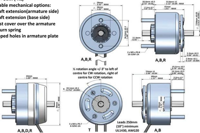
Data at 20°C, device connected to heatsink 310x310x3mm aluminum return spring 45 ~ 65 mNm
