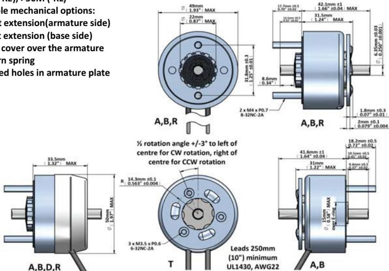
½ rotation angle +/- 3° to left of centre for CW rotation, right of centre for CCW rotation
