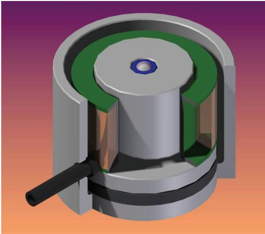
HMER devices incorporate a permanent magnet so that high holding force is developed to a flat ferromagnetic component without external power being applied. Power is applied to the device with reverse polarity to counter the field due to the permanent magnet and release the 'keeper' component.
