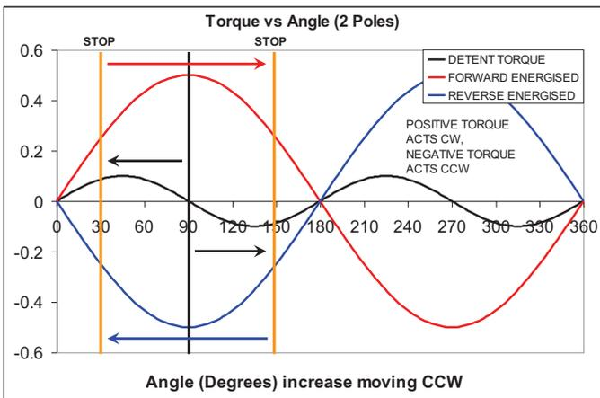
points (which are zero torque points), they should restrict motion to a region where developed torque is sufficient to turn the load at required speed, or to hold the load. For more efficient operation, shape of the torque curves may be modified to optimise behaviour for a particular rotation angle.
