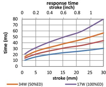
Data at 20°C, device connected to heatsink 150x150x3mm aluminum
