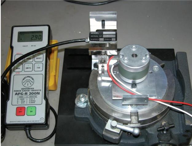
the part energised from a regulated current source. Current regulation stabilises the response time of the solenoid against variations in supply voltage or operating temperature. The solenoid is energised with specified current condition, and is rotated whilst monitoring torque output to derive the torque curves. The torque is measured turning in either direction, and the lower of the two measured
