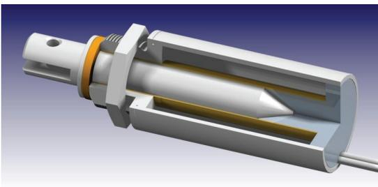
Both the open frame solenoid, and the tubular solenoid, employ a construction in which the plunger slides directly in the sleeve of the solenoid, which may be a brass or stainless steel sleeve, or in some cases the plunger may slide directly in the
