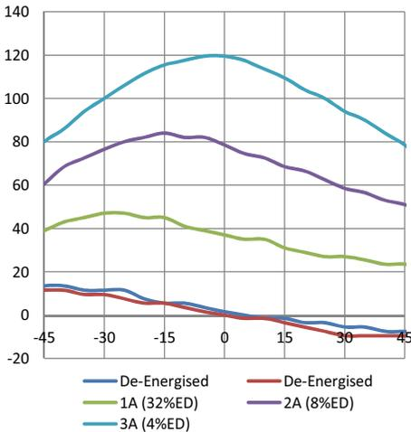
Response (ms) vs Load Inertia ( $\text{gcm}^2$ )
