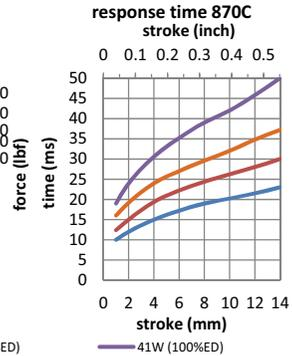
Data at 20°C, device connected to heatsink 520x520x3mm aluminum
