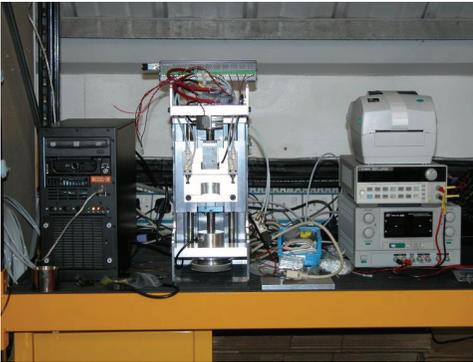
We have designed and developed in-house test systems for characterising force and displacement behaviour of devices for several years, recent developments in this area include digital force transducers to reduce the noise inherent to analogue sensors (valuable for hysteresis measurement where hysteresis values may be <0.1% of measured force values).
