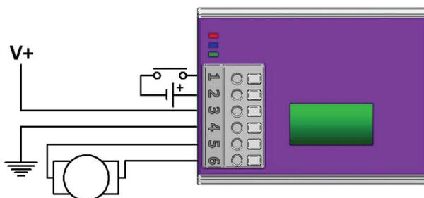
The load is connected between terminals 5 & 6.
