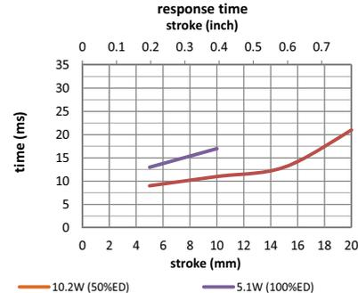
Data at 20°C, device performance measured without heat sink
