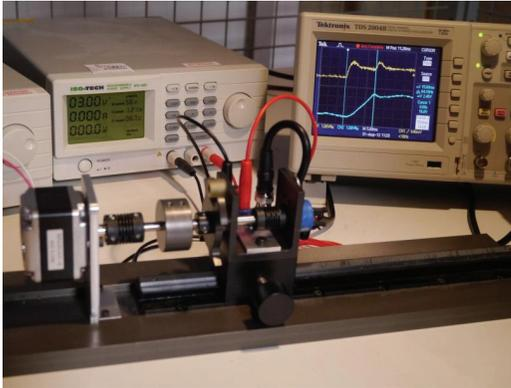
response speed data is the source voltage from which the current regulator works. The measured performance corresponds to the behaviour that will be achieved with excitation at the nominal voltage when the coil temperature is elevated to approximately 80°C. It should be noted that the source voltage influences the rise-time of the current to reach rated value – a high source voltage will enable shorter electrical rise time and faster actuation times.
