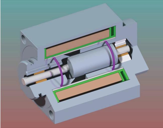
face of the solenoid to the base pole piece. The image shows a proportional solenoid which is constructed in this way. In this case the device is shown as having o-ring seals sealing the front and rear pole pieces into a metal tube,
