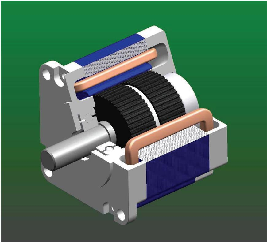
The large number of sub-poles also means that the polarity of the magnetic field in each pole must be reversed many times to complete revolution, as the speed of rotation, and frequency of these polarity reversals increases, magnetic losses in the stator assembly increase. This limits the maximum rotational speed of stepping motors.
