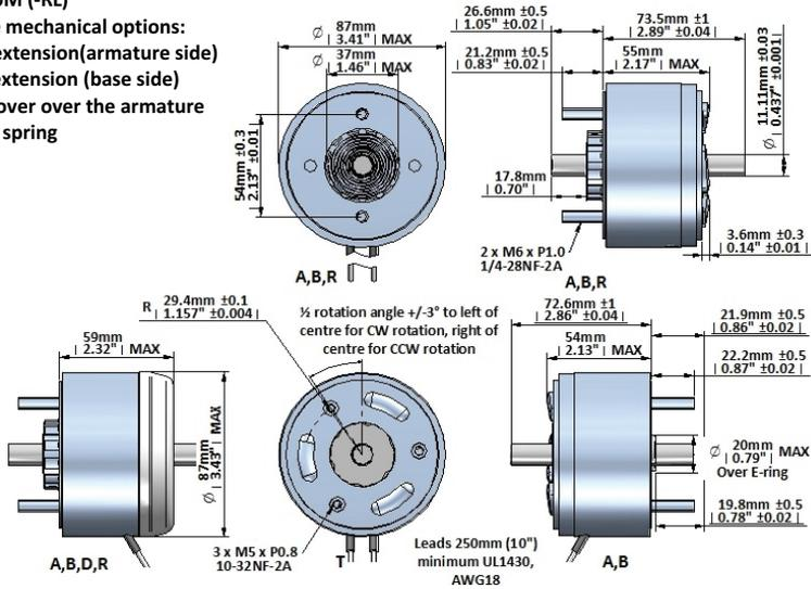
Data at 20°C, device connected to heatsink 520x520x3mm aluminum return spring 90 ~ 140 mNm
