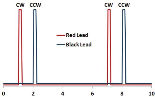
By closing either S1 and S4, or S2 and S3 while the other switches are open, the current can be caused to flow through the solenoid coil in either the forward or the reverse direction. With momentary excitation pulses as depicted in the timing diagram the solenoid can be pulled in or released, remaining in either position with no power applied in between.
