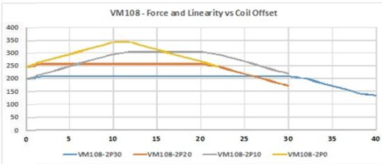
The VM108-2P voice coil motor can be configured with different coil geometry to provide more force over a shorter linear range. The graph gives an approximate indication of what is possible. Call Geeplus if other
