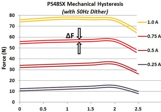
If the force developed by the solenoid is measured in a fixed position as the current is increased, another curve can be plotted which is a loop as shown, the force difference between upper and lower curves in this case represents (mostly \*) magnetic hysteresis caused by losses in the magnetic steel material.
